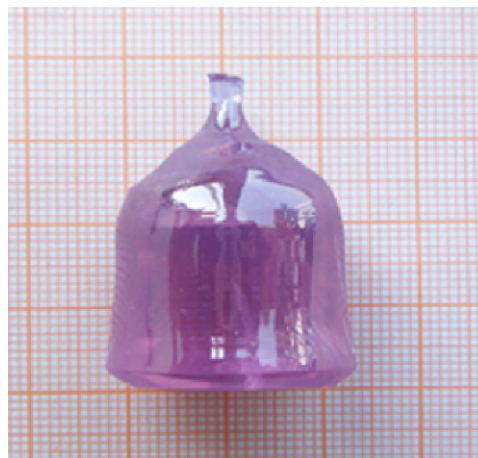
Fig. 3. \text{Nd}^{3+}:\text{Na}_2\text{Gd}_4(\text{MoO}_4)_7 crystal grown by the Czochralski method (where white color is reflecting light).
